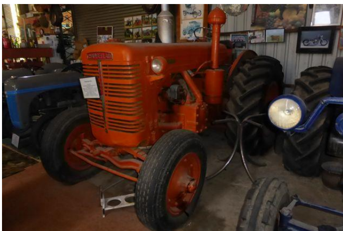
Chamberlain tractor with opposed engine (Kev's Kollection)
