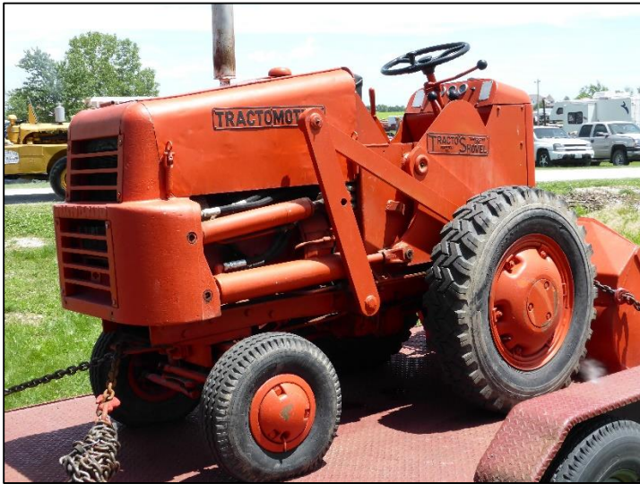
TL-B loader with a 'B' tractor powertrain. One of 65 built.
