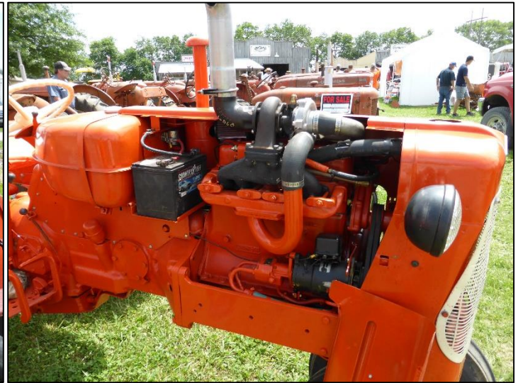
Modified D-15 diesel (turbo added).
