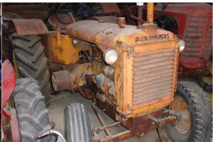
A-C 'U' with unique rad shutters (Kev's Kollection)
