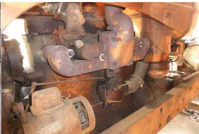
Unique dual fuel manifold on a WD-45 (Roger Griffin collection)
